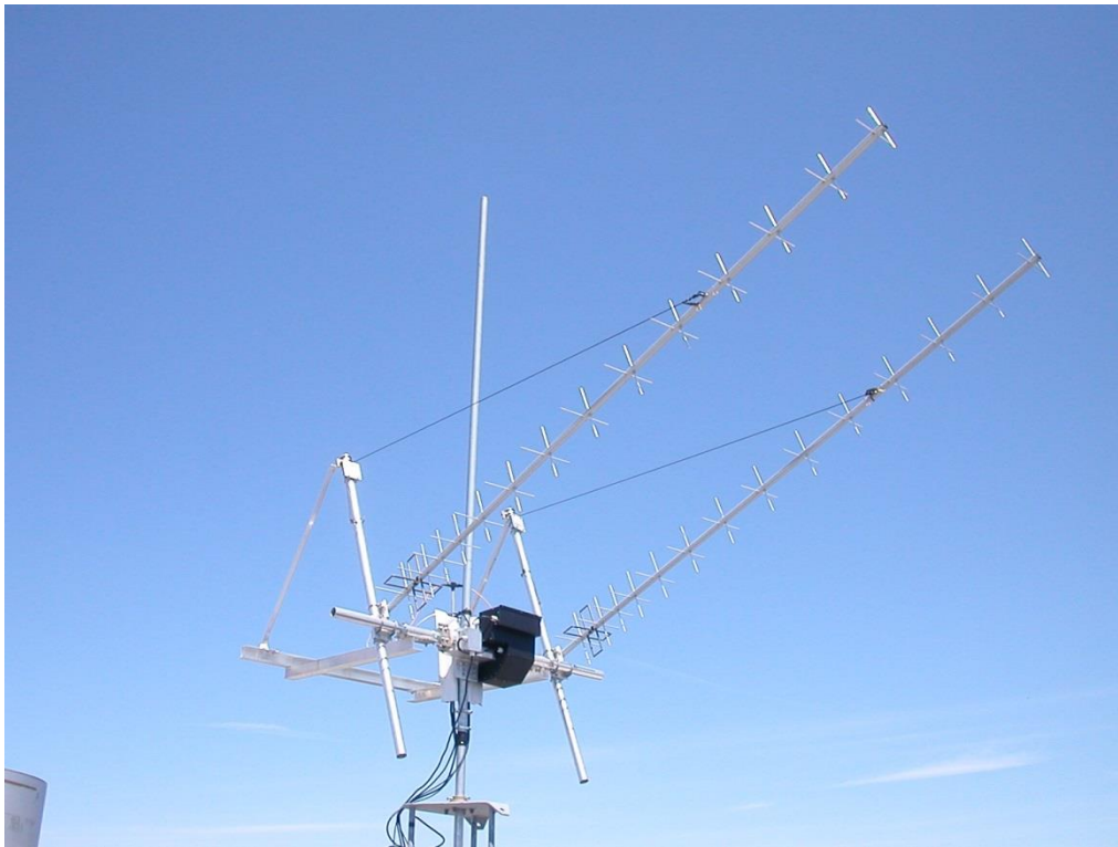
Fig 2. – A pair of 15LFA-JT rear-mounted Yagis on a simple mount with azimuth and elevation control. Light-duty Dacron ropes serve as forward guys, to prevent boom sag.
