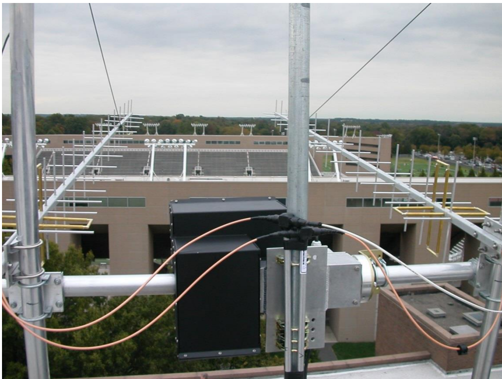
Fig 3. – Separate feedlines carry signals for horizontal and vertical linear polarization from each Yagi to the power splitters.
