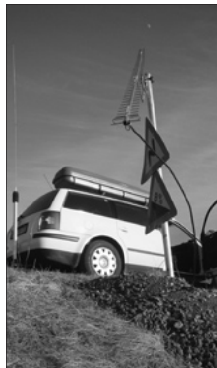
Fig 30.66 — TF/DL3OCH used a rural road sign to help him give contacts with Iceland to a number of EME operators on 1296 MHz. Bodo has activated many DXCC entities on 1296 MHz EME by using JT65, a single long Yagi and a 100 W solid state amplifier.
